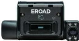
Dual facing dashcam. Integration of dashcam with Ehubo data and other key driver and vehicle statistics supports advanced driver coaching and accident exoneration in MyEROAD Replay.
